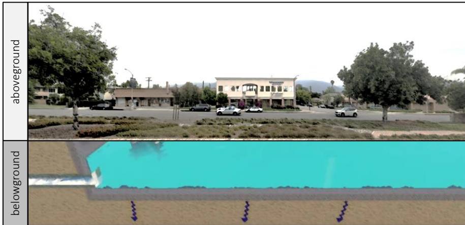
Underground regional infiltration system below a street median
