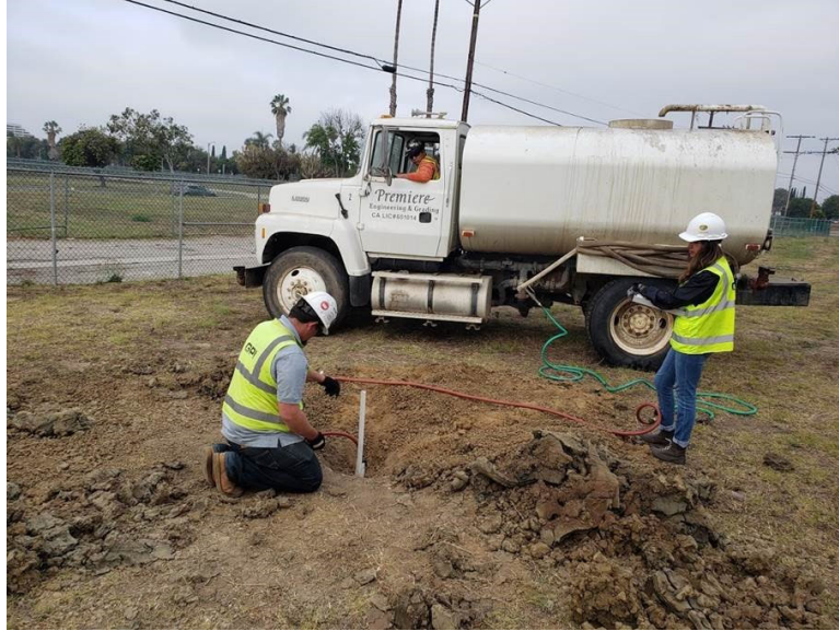
Well permeameter test being conducted at LAX project.
