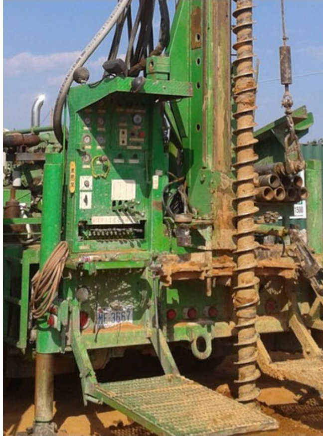
8" hollow stem auger typically used for infiltration tests.
