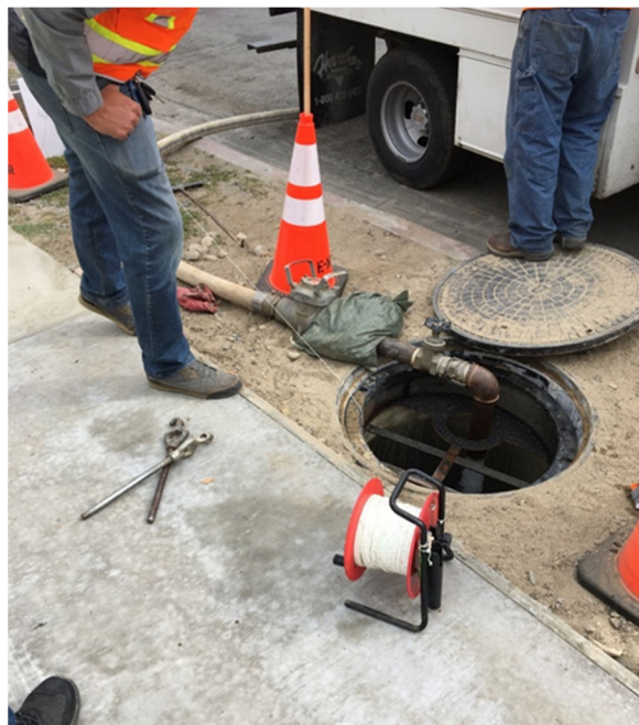
City of Los Angeles (North Hollywood) full-scale drywell percolation test
